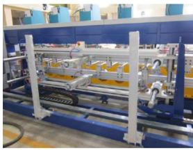
The concept of fixturing for geocell welding system is that it needs a rigid base wherein the pneumatic press comes down and welds each geo in a sequential operation. The number of fixture rods depends on the number of heads & the sequential operation that needs to be carried out.
