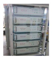
The SG-22 series generator has amplitude regulated power system with LED display of output power, amplitude, overload indication and frequency. It has a potentiometer to control the amplitude manually. It is staked as per the quantity. The output power of the generator is 3000W/ 4000W/4500W.
