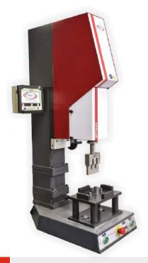
As a joining process for industrial thermoplastics, the ultrasonic method is very well proven in practice. Particularly in the production of mass- produced parts, the process offers definite advantage over previous methods such as for instance high strength, clean weld seams, fast processing times, extremely low rejection rates and low energy consumption.
