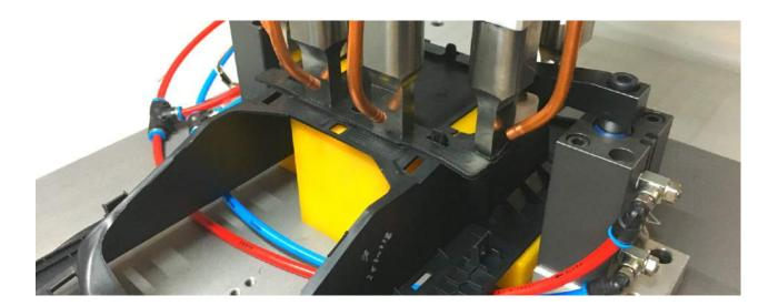
For Large/Complex components, system with multi converter design (with mother / daughter horns) are available as per specific requirements. Multi-converter units are frequently used in the welding of large area, asymmetrical parts, for example in automobile and apparatus engineering or with toys. The advantage of multi-converter system lies in the construction of small, simple Sonotrodes/Horns which facilitates to optimise the weld quality along the whole weld contour due to local targeting.
