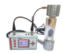
UCT is a fully portable instrument for assessing the strength of concrete either in situ or precast. It complies with the British Standard BS -4408 (Part V – 1974), BS-1181 and ASTM C-597. It is designed with field conditions in mind and is very simple to operate. Its accuracy and stability are unmatched. It generates low frequency pulses and measures the time of flight in the material. The time is displayed by 5 digit display.
